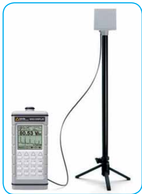
Fig. 17 - Measurement Kit consisting of palm PMM8053 and sensors EHP50C, for measuring up to 100 kHz, and EP330 for frequencies up to 3 GHz.
